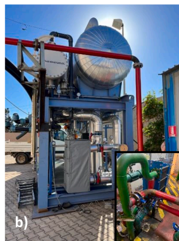
Fig. 2. A) block flow diagram of the heat input section of the med prototype plant. b) picture of the inlet heat exchanger and flash drum (inset showing the connection with the engine cooling circuit for waste heat recovery).
