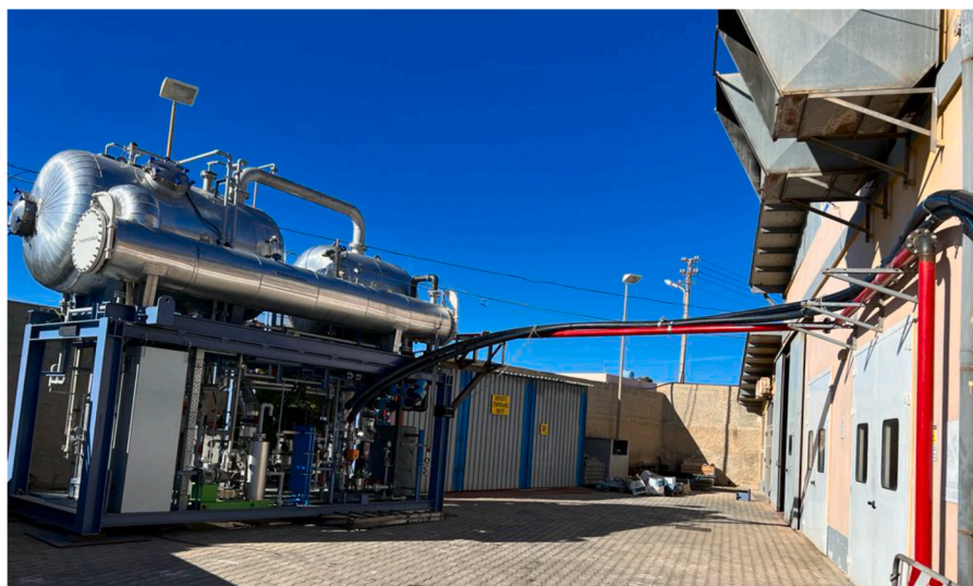
Fig. 1. A) block flow diagram of the med prototype plant representing the main units constituting its 4 sub-sections. b) overview picture of the med pilot with the interconnection pipes conveying hot water from the engine and cooling water for the condenser.
