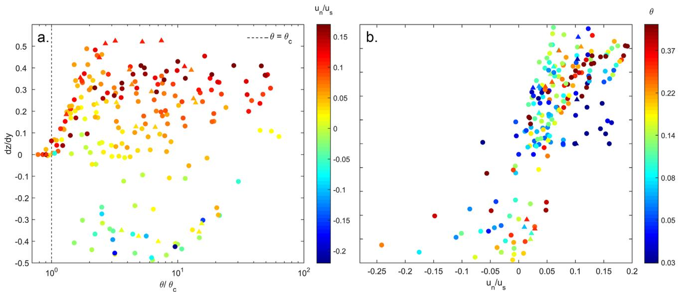
**Figure 7.** Average transverse bed slopes of all experiments. (a) Transverse slope against relative sediment mobility. Color scale indicates secondary flow intensity and direction. (b) Transverse slope against secondary flow intensity. Color scale indicates sediment mobility.
