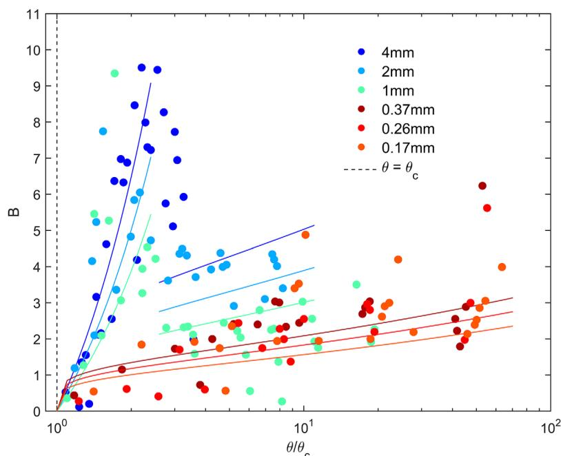
**Figure 11.** Empirical fits to experimentally determined slope factors as a function of relative sediment mobility and grain-size. The fitted functions have a similar shape as existing relations found in literature (equations (11) and (12)).
