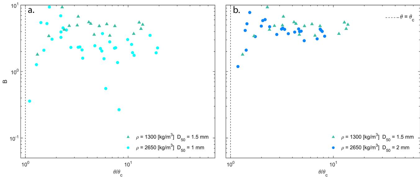
**Figure 9.** Trend in slope factor ( $B$ ) against relative sediment mobility for experiments with low-density sediment, compared with experiments with normal sediment with median grain sizes of (a) 1 mm and (b) 2 mm.
