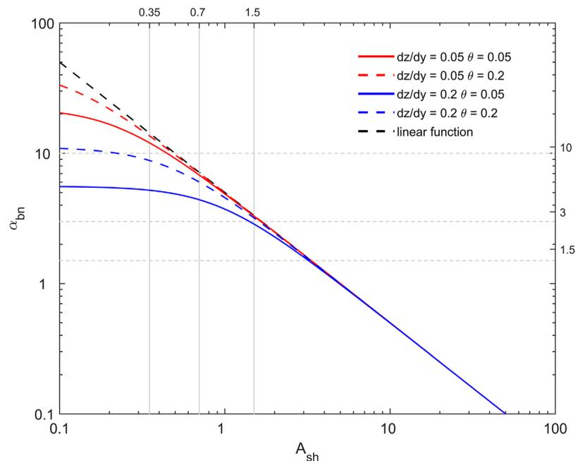
**Figure 14.** Relation between  $\alpha_{bn}$  and  $A_{sh}$ , the input parameters of the two main options to calculate sediment transport on transverse bed slopes in the morphodynamic model Delft3D (equation (B1)). Colored lines indicate different combinations of transverse slope and sediment mobility, with a critical sediment mobility of 0.04. Gray lines indicate frequently used input parameters as described in section 2 and used in Figure 12.
