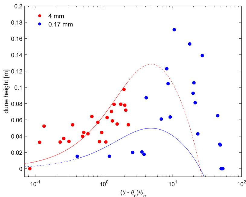
**Figure 13.** Comparison between the dune height observed in the experiments with a median grain size of 4 and 0.17 mm (scatter) and the dune height as predicted by Van Rijn (1984b) (lines). Solid lines represent the predictor for relative sediment mobility in the range of the experiments, while dashed lines show the whole trend of the dune height predictor from lower stage plane bed to upper stage plane bed.
