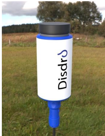
Picture 1 Disdro sensor. Acoustic disdrometer measuring rainfall.
