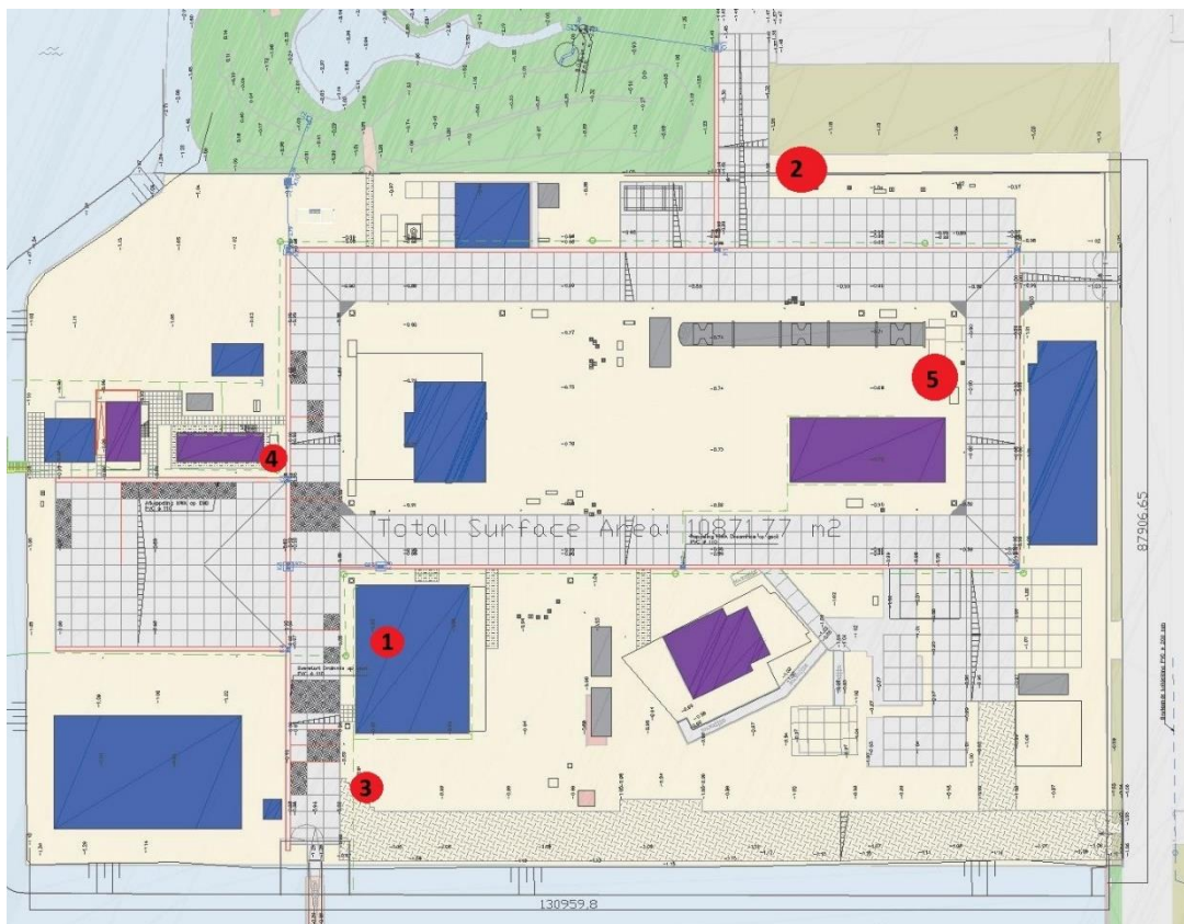
Figure 18 Locations of the sensors on WaterStreet, the study area. The groundwater sensors, weather station, and KNMI station location can be seen in this figure. These sensors are the ones found until April 2021.
