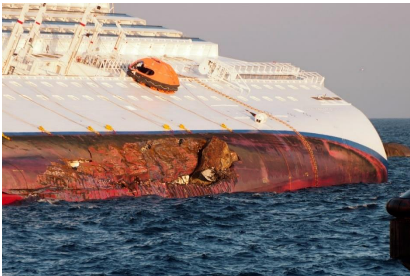
Figure 3 Damage to the hull
