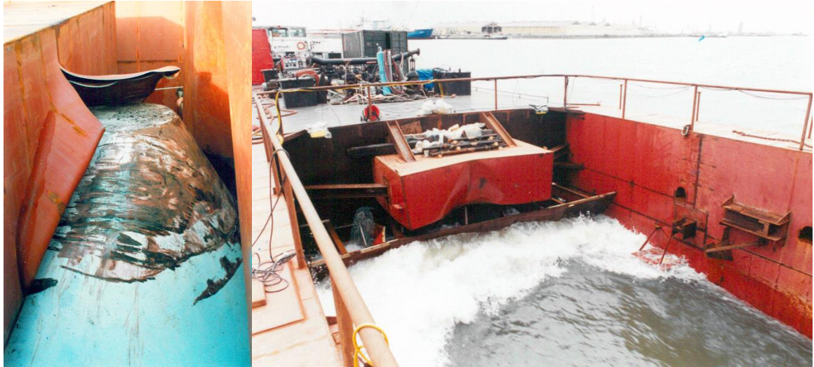
Figure 16 Left: The artificial rock stuck in between the test-section and the buffer. Right: The damage to the buffer by the rock after removal of the test-section.
