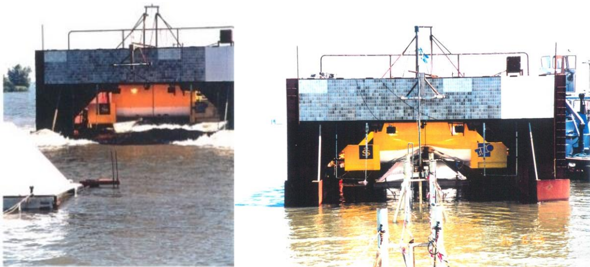
Figure 6 Left: just before grounding, approaching the rock at approximately 7 kts. Right: Just after grounding. Rock stuck in buffer.
