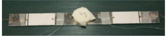
Figure 2: The traveling wave piezoelectric beam robot, courtesy of Hariri et al. [23]
