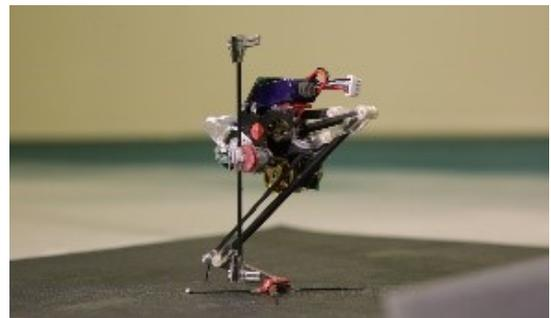
Figure 12: The singular jumping robot SALTO, courtesy of Haldane et al. [83]
