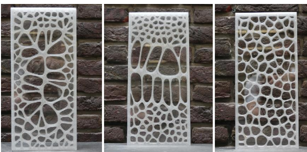
Figure 3. Glass panels (3D-printed PETG Voronoi core) (Neeskens, 2018)
