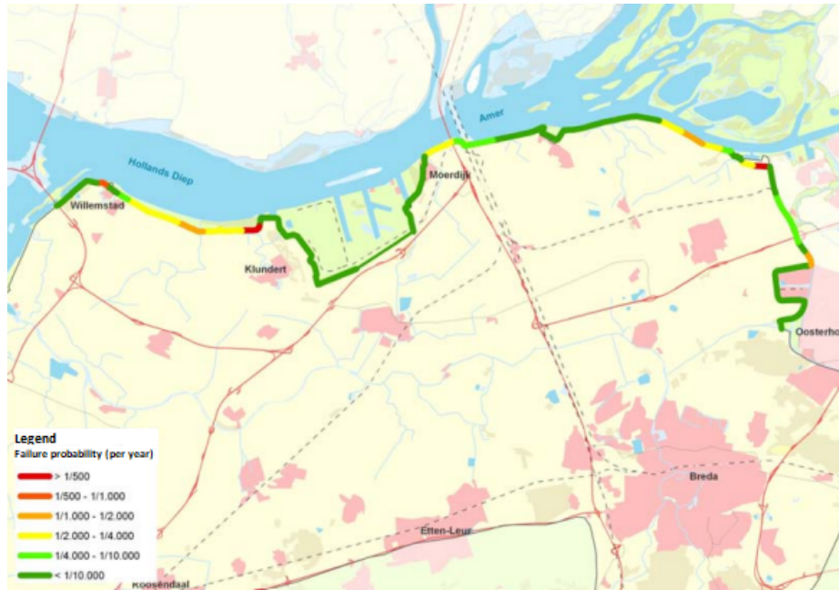
Figure XII.3: Failure probabilities dike sections West-Brabant (modified from Arends and Nieuwhof (2011))
