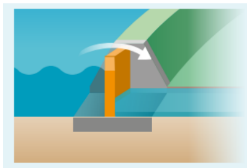
Figure 5.20: Failure mechanism of overtopping (Onwuachu, 2021)
