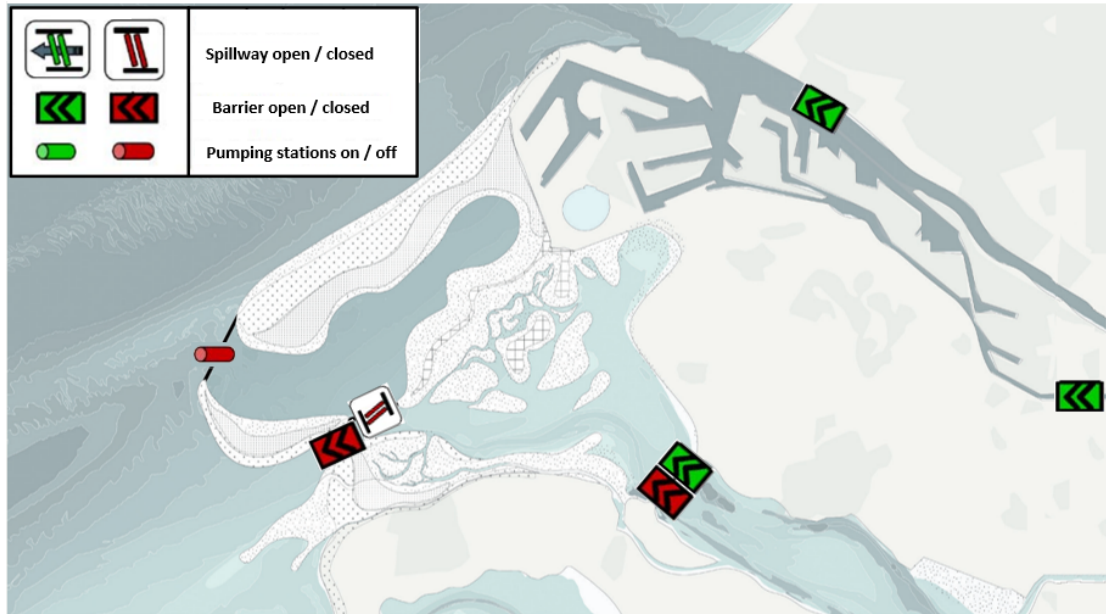
Figure IV.13: Water management system during scenario 3.1 (modified from van Eeden (2021))
