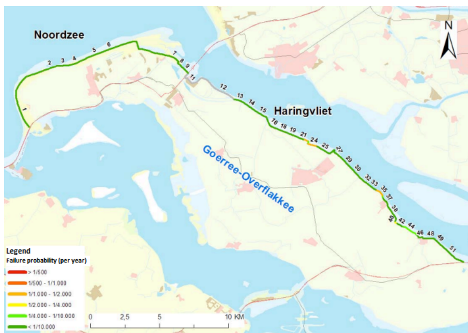
Figure XII.2: Failure probabilities dike sections Goeree-Overflakkee (modified from Bisschop and Karimlou (2014))
