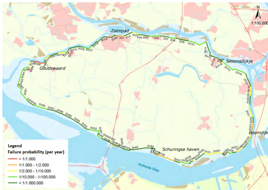
Figure XII.4: Failure probabilities dike sections Hoeksche Waard (modified from de Groot (2014b))
