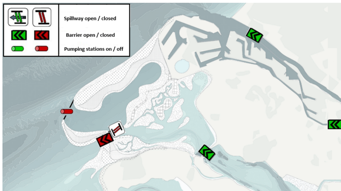
Figure IV.3: Water management system during scenario 1.1 (modified from van Eeden (2021))
