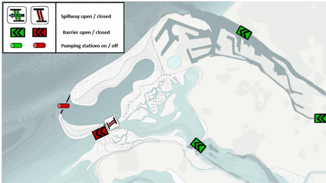
Figure IV.7: Water management system during scenario 2.1 (modified from van Eeden (2021))
