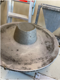
(a) B2 slump test
