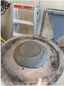
(b) B2 spread test
