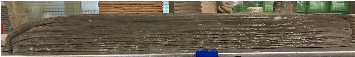
Figure 6.6: B3lbA0.5 Printed Wall
