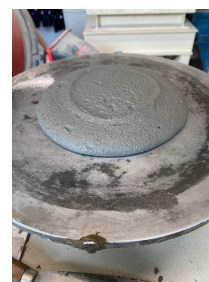
(b) B1.5 spread test
