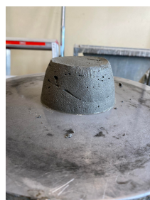
(a) B1.5 slump test
