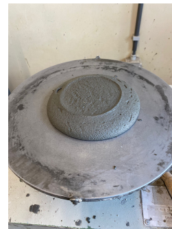
(b) B3CM1 spread test
