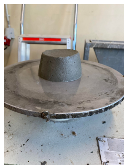
(a) N4A0.75 slump test
