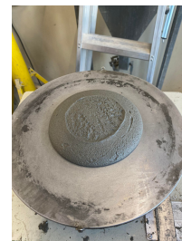
(b) B3A0.75 spread test
