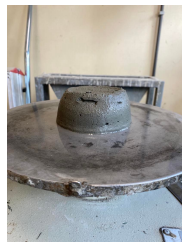
(a) N4 slump test
