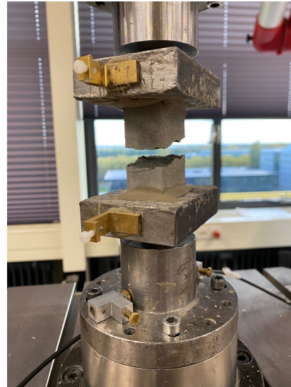
(b) Setup of the Test with a sample after failure
