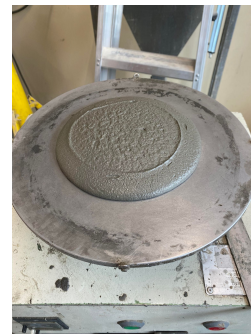
(b) B3X0.2 spread test
