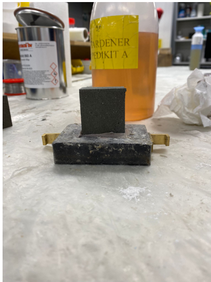
(a) Sample for tensile bond strength glued to the metal place from one side
