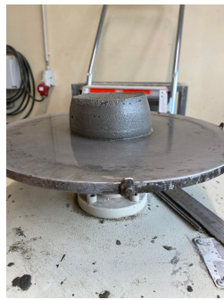
(a) B3X0.2 slump test
