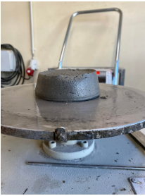
(a) B3 slump test
