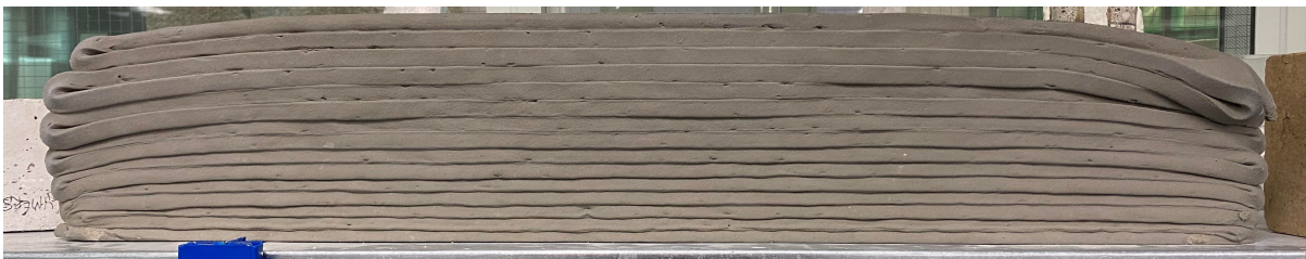
Figure 6.7: RefA0.75 Printed Wall
