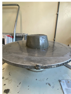
(a) N4CM1 slump test
