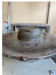
(a) Ref slump test
