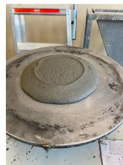
(b) N4A0.75 spread test
