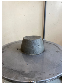
(a) B3CM1 slump test
