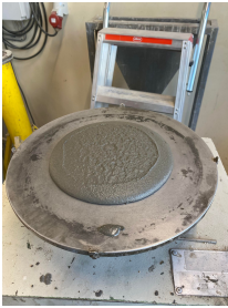
(b) B3 spread test
