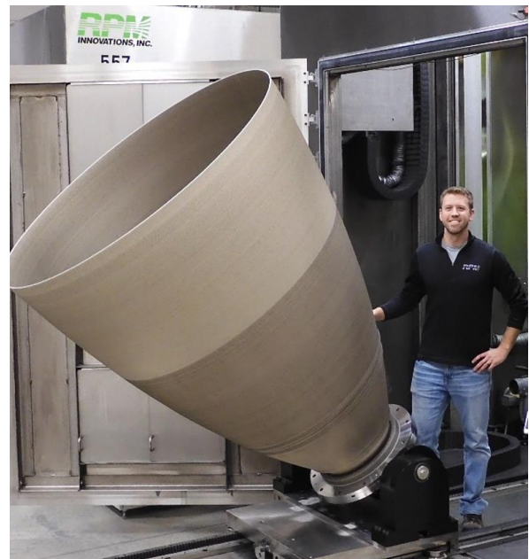
Figure 2. Large-scale LP-DED integral channel nozzle manufactured with LP-DED in 90 days (1.52 m dia. and 1.78 m height).
