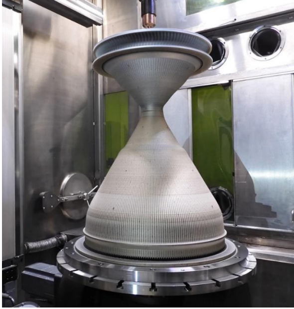
Figure 3. Example of a combustion chamber liner built using LP-DED with internal channels.
