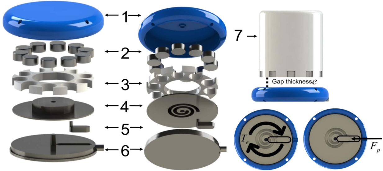
Fig. 5. 3D-model overview of the actuator component of the prototype and the working mechanism. 1) PEEK hood, 2) neodymium magnets, 3) 3D-printed magnet holder, 4) 316L Stainless Steel (SS) spiral, 5) 316L SS pin and follower, 6) 316L SS backplate and groove for the follower, and 7) external magnets used to apply torque T_e to the actuator through an identical set of magnets. Upon rotating the external magnets, the actuator magnets rotate and guide the pin through the spiral in 1 linear degree of freedom through the groove in the back plate to generate output force F_p non-invasively through a gap thickness of e . Models were made in SolidWorks (Dassault Systèmes, Paris, France).
