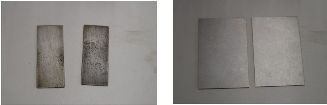
Figure A1: Fe-electrodes used for EC in batch studies (left) and in the filtration columns (right)
