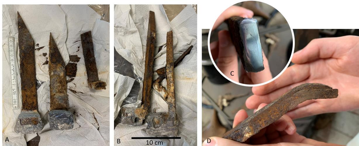
**Figure 4.3:** A and B) The anchors from the Domtoren. C) The cross-section of the anchor with a long slag inclusion running through the length. D) The bent tip of the anchor shows the split of the two piling layers.
