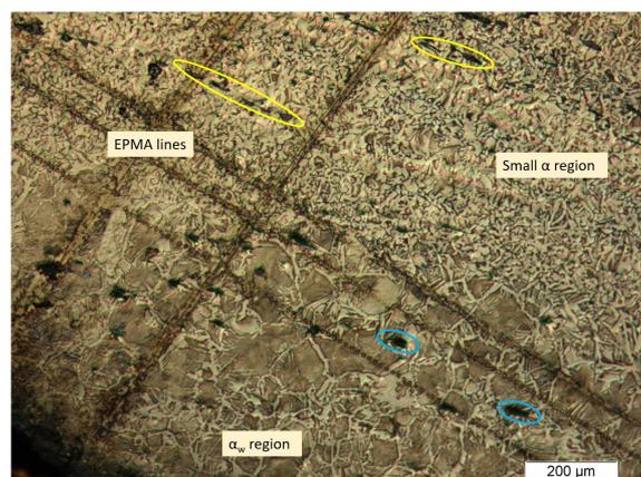
**Figure 5.2:** OM of H-CS-8, showing the Widmanstätten microstructure near the surface of the sword, ferrite and pearlite alternating grains, the measurement lines of the EPMA and two types of slag inclusions. (blue: glassy. Yellow: wüstite-glassy/fayalite)
