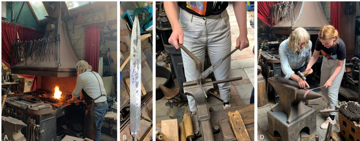
**Figure 4.4:** A) The blacksmith's fire. B) The mock-up sword before bending. C) Bending the cold sword with a leverage effect. D) Bending the reheated sword by hammering.
