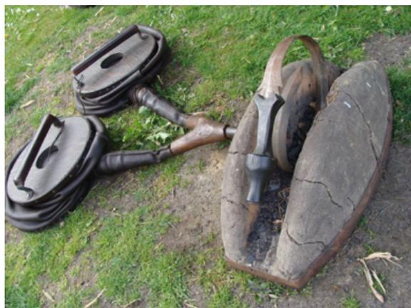
**Figure 4.2:** Furnace designed by Thijs van de Manakker for bending the replica of the sword of Oss. Photo by Thijs van de Manakker.
