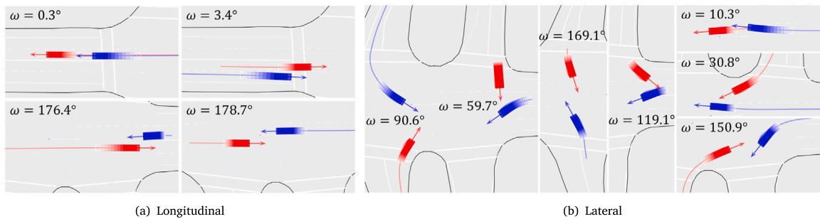
Fig. 1. Real-world examples of vehicle interactions in urban environments. \omega is the angle between moving directions of the interacting vehicles. (a) Vehicle interactions only in the longitudinal direction. (b) Vehicle interactions involving both longitudinal and lateral directions.
