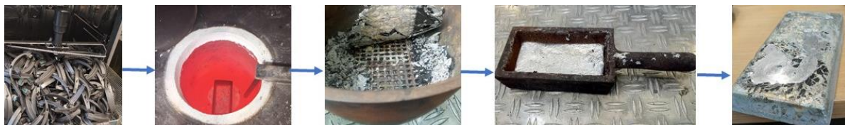
Figure 2. “All in One” process on one location.
