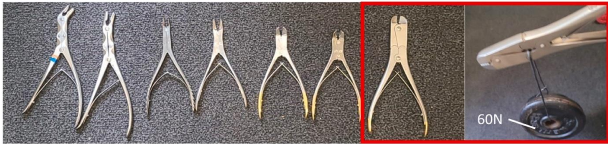
Fig. 4. Testing bone cutting hinge force. Left, tested bone cutters ordered from low to high hinge force. Right, bone cutter with highest hinge force opens when loaded with 6 Kg mass.
