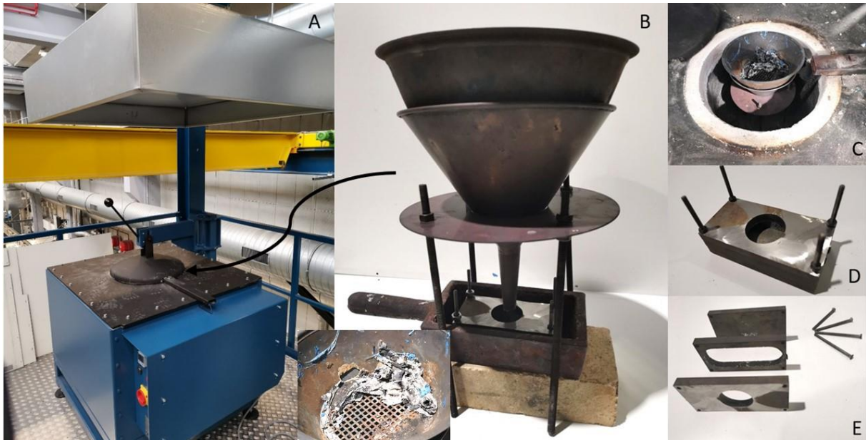
Figure 3. Melting Oven. A: The induction furnace for melting of the Zamak laryngoscope blades. B: All-in-one casting setup, a bowl with grate placed in the melting oven. C: Top bowl with filter allows only the Zamak to pass. D: Cast with riser. E: Exploded view cast with riser.
