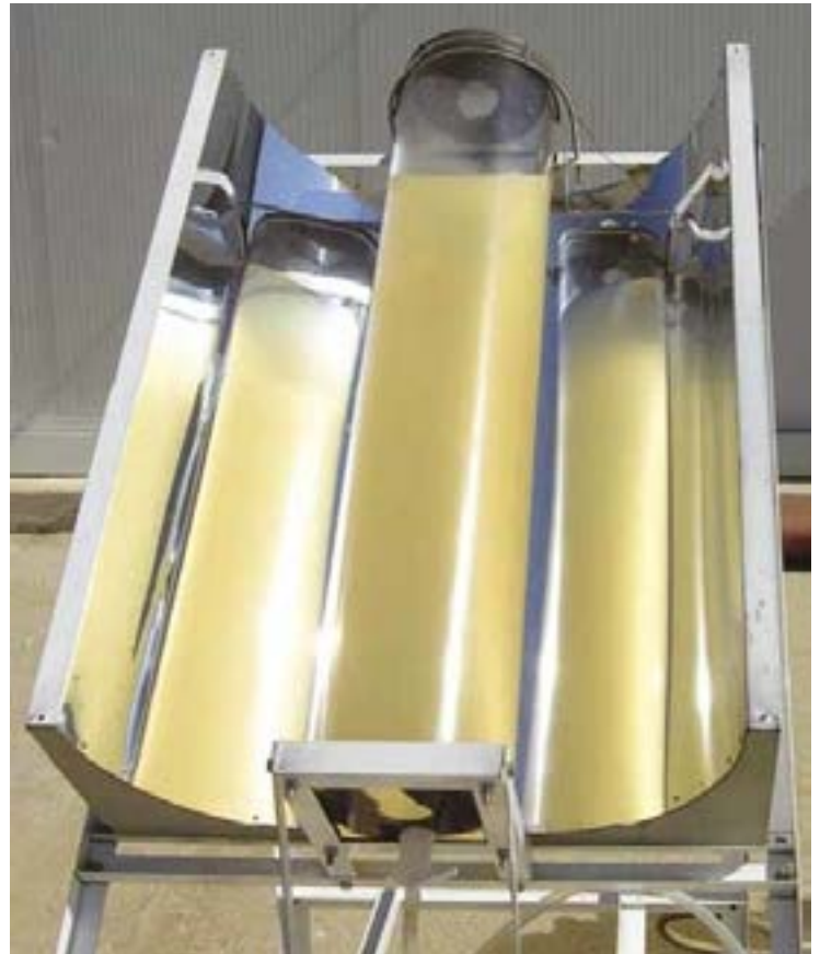
Figure 16. Solar Disinfection tube combined with a Compound Parabolic Collector (Ubomba-Jaswa et al., 2010). The tube holds 25 L.
