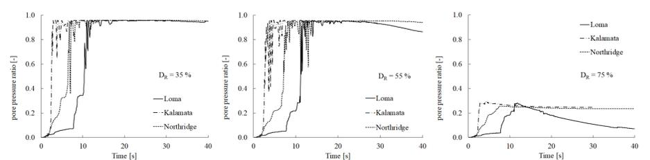
Figure 3 - Comparison of the pore pressure ratio evolution for loose (left) and medium loose (center) and dense (right) sand, for different earthquake recordings.
