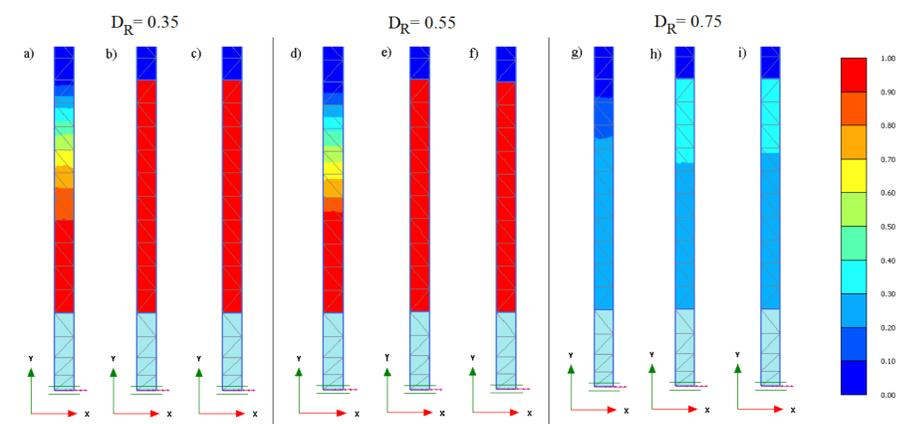
Figure 2 - Maximum pore pressure ratio contours for Loma Prieta earthquake (a, d, g), Kalamata earthquake (b, e, h) and Northridge earthquake (c, f, i) for different relative densities.
