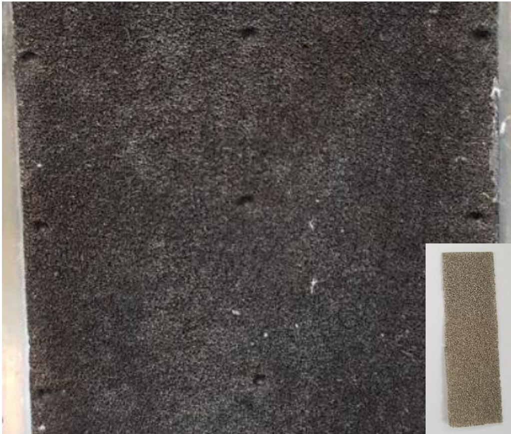
Figure 14: Cathode after the experiments were carried out. Original nickel foam material in the bottom right.
