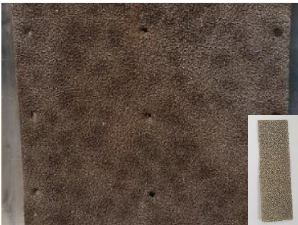
Figure 15: Anode after the experiments were carried out. Original nickel foam material in the bottom right.
