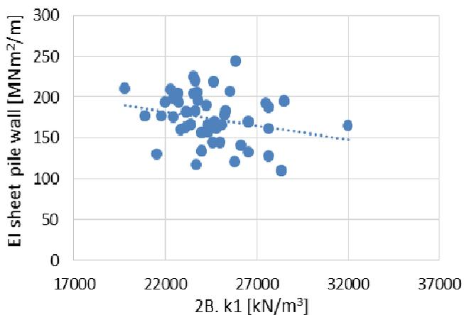
Figure 9. Possible parameter input combinations with same displacement as outcome as found for calibration of phase 3.
