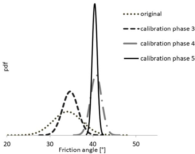
Figure 8. Calibrated friction angle of layer 2B.
