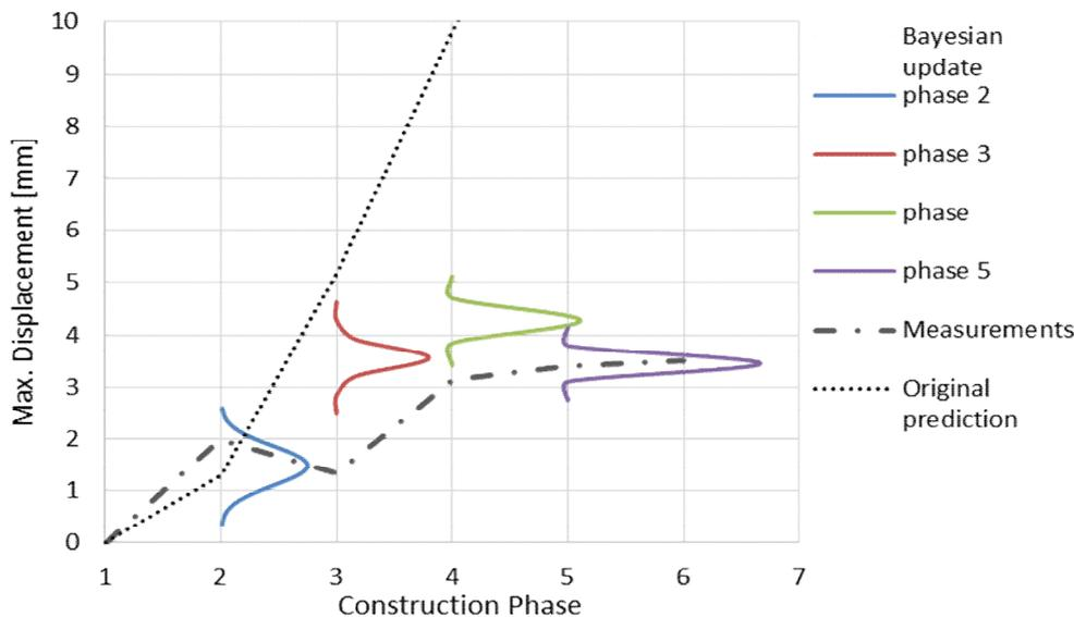
Figure 6. Bayesian update for construction phases 2-5.
