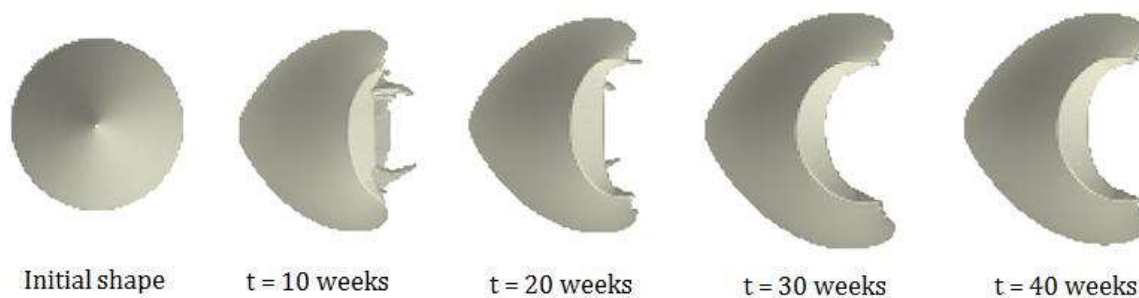
Fig. 4. Formation of a barchan dune from a cone-shaped topography with wind velocity of 6 m/s.
