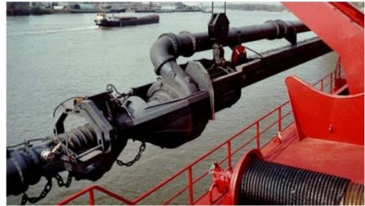
(b) UWP located between upper and lower suction pipe, source = (IADC, 2022)
