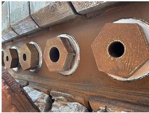
Figure 2.10: Varying jet nozzles diameters of TSHD: HAM 318
