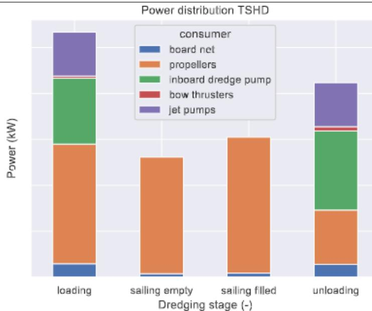
Figure 1.2: Power distribution results of study by: (van der Bilt, 2019). Power distribution is plotted for different energy consumers based on empirical coefficients
