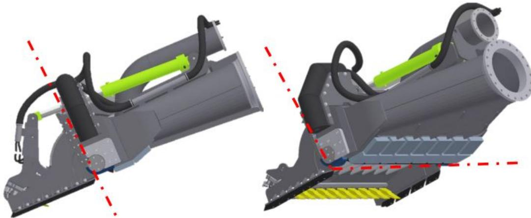
Figure 2.5: Side view of draghead configuration with a hydraulic cylinder, source: (ter Meulen, 2018). The left part of the red line is the visor, the right part is the draghead house.
