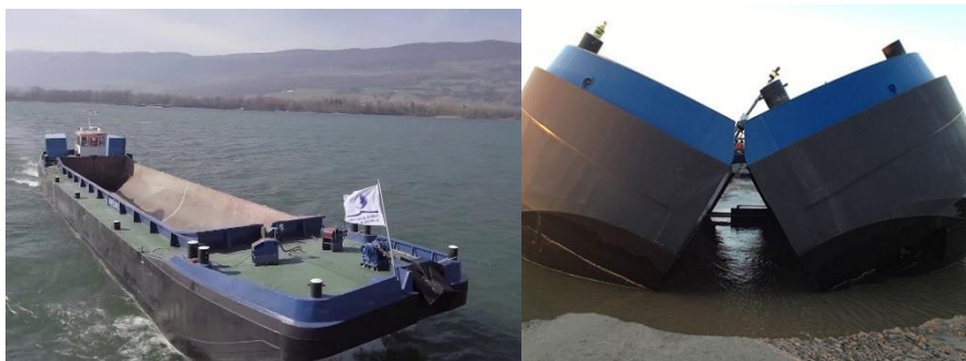
Figure D3: Barge split hopper while navigation (left), at use (right)
