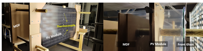
FIGURE 5 The setup was built according to the physical properties of the PV module used. Left, the setup without the front glass. The thermocouples were installed in the geometrical middle of the setup, as is also shown in Figure 6. Right, the full setup with front glass and the plastic side coverage sheets. PV, photovoltaics [Colour figure can be viewed at wileyonlinelibrary.com ]
