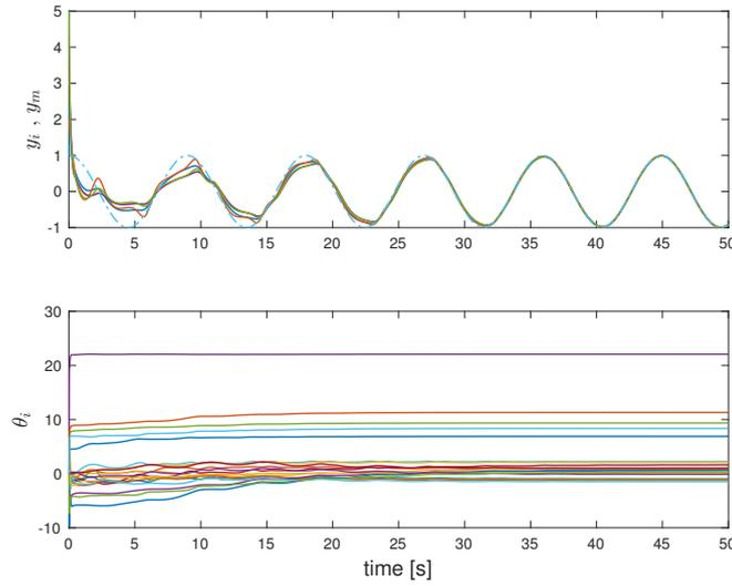
**Figure 3-4:** Synchronization of the outputs of each agent  $i$  to the leader output using (3-42), and corresponding adaptive gains.
