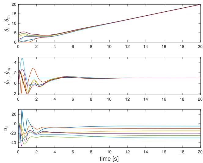
**Figure 5-5:** Protocol (5-27): synchronization of the states of each agent  $i$  to the reference state  $[\theta_m, \dot{\theta}_m]$ . The control inputs  $u_i$  are shown at the bottom.
