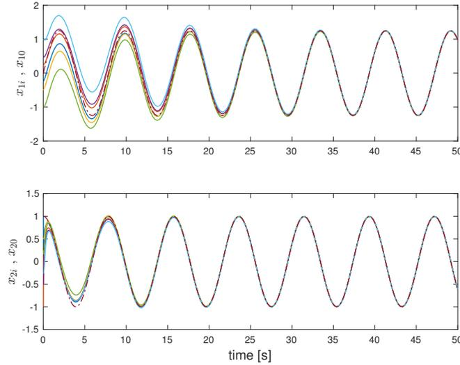
**Figure 4-2:** Synchronization of the states of each system to the leader reference state using (4-16) and (4-17).
