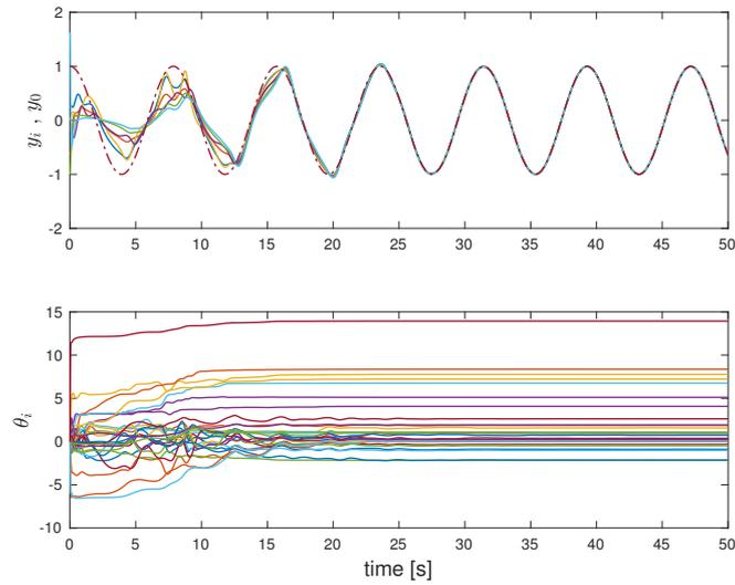
**Figure 4-4:** Synchronization of the outputs of each system to the leader reference output using (4-36), and corresponding adaptive gains.
