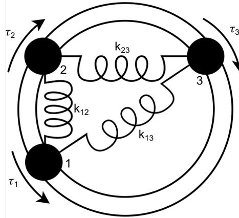
**Figure 5-1:** Mechanical analogy of a network of three coupled oscillators.
