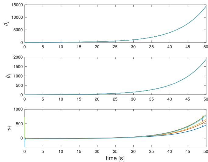
**Figure 5-8:** Leaderless synchronization of the states of each agent  $i$  using protocol (5-14). The control inputs  $u_i$  are shown at the bottom.
