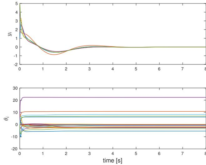
**Figure 3-5:** Leaderless simulation: synchronization of the outputs of each agent  $i$  using (3-42), and corresponding adaptive gains.
