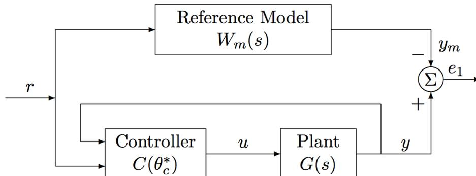
**Figure 2-2:** Structure of MRC scheme [Ioannou and Sun, 2012].
