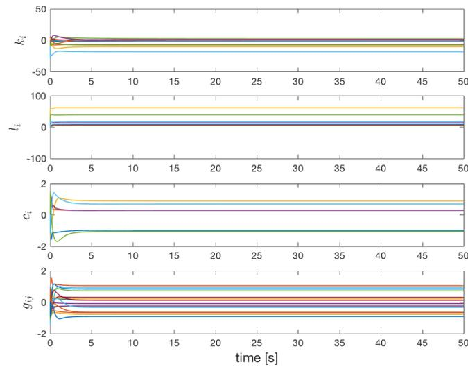
**Figure 5-9:** Leaderless synchronization using protocol (5-14): adaptive gains.
