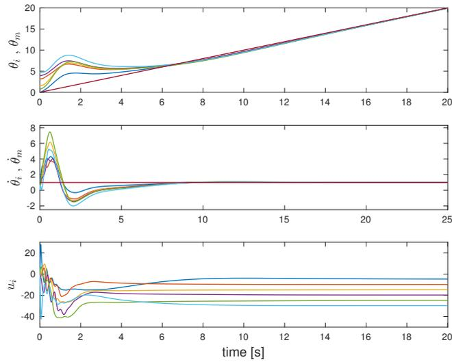
**Figure 5-3:** Protocol (5-14): synchronization of the states of each agent  $i$  to the leader reference state  $[\theta_m, \dot{\theta}_m]$ . The control inputs  $u_i$  are shown at the bottom.
