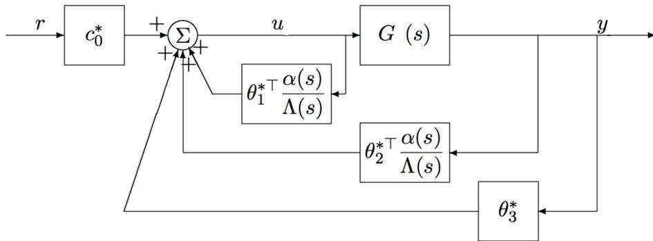
**Figure 2-3:** MRC architecture using controller (2-12) [Ioannou and Sun, 2012].
